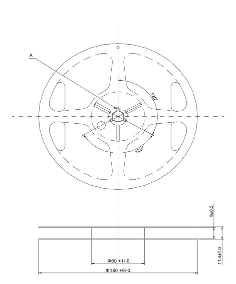
Material:Polystyrene (Conductivity) unit:mm
